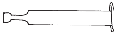
ea. - Cam Pins push through holes in panels. (Side, Back, and Bottom Panels)
